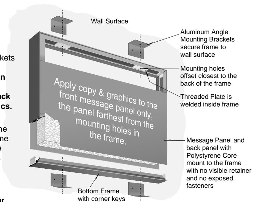
Signs ship completely assembled ready to be installed with the supplied angle brackets.
